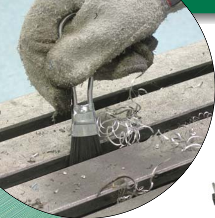
← Removing hot chips from the slots of a milling machine.
