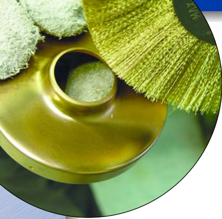
Producing an antique finish on a brass door knob rose.
