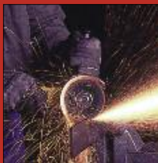
Notching a steel bar prior to welding.
